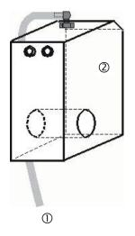
➤ If water sprays from the vent hole ① of the measuring chamber ②, reduce the amount of inlet water via the manually operated shut-off valve. It should take 2 to 6 seconds to fill the measuring chamber!
