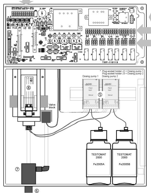
Terminal block for inputs Start, Stop, IN1, IN2, and output OUT
